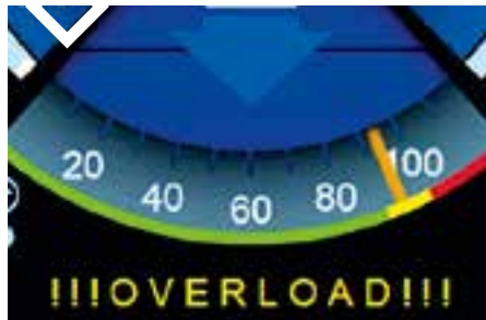
OVERLOAD WARNING DEVICE*
